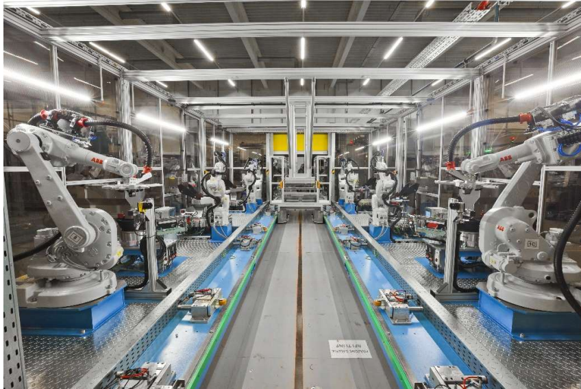
Photo 1: A view inside the machine of the robots that are tasked with assembling screws and clips
