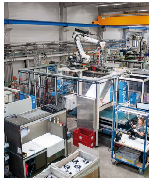
Production cell for the decorative strip: 2C injection moulding machine GXL 651-3000/750 with rotary table and six-axis robot for film and part handling.
