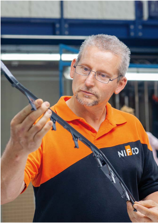
Joachim Schinke, head of the injection moulding department, inspects the decorative strip, which is challenging in terms of gap dimensions and surface.
