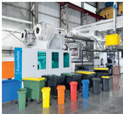
Colorful variety: Weber produces large volume waste disposal containers in a variety of shapes and colors on the MXH 5500.
