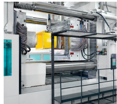
The custom solution allows safe handling of the molds, which can weigh up to 150 t.
