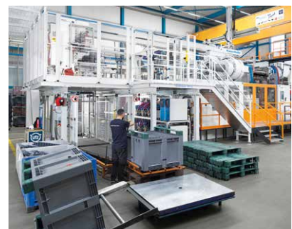
The two-story automation completes the following process steps, such as the application of RFIDs, IML barcodes and logos, plus post-mold processing and partial quality control
