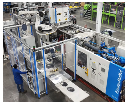
Thermoplastic lightweight construction for large-scale production: The GXW 450-2000/1400 with swivel platen
