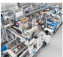
High degree of automation: All eight injection molding machines are equipped with LRX linear robots from KraussMaffei
