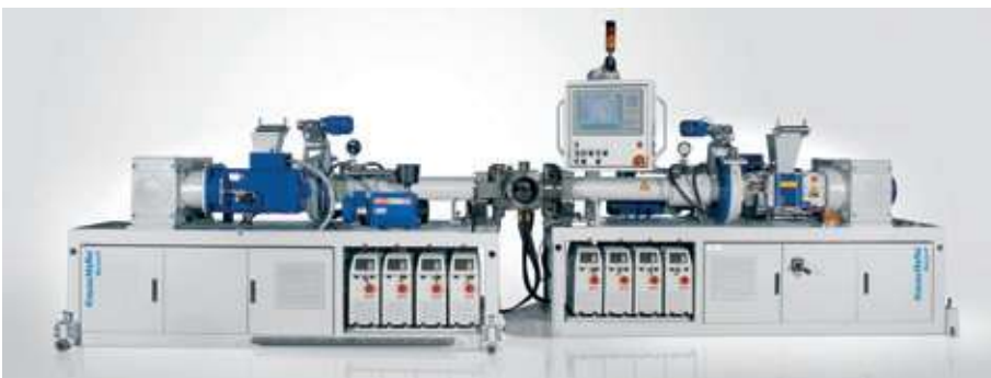
Two Pinconvert extruders for manufacturing a multi-component profile
