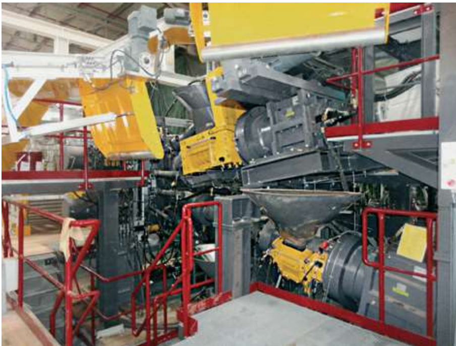
GE-W hot-feed extruders – best suited for co-extrusion systems
