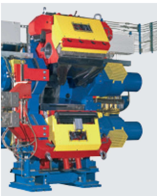
Hydraulically adjustable duplex extrusion head
