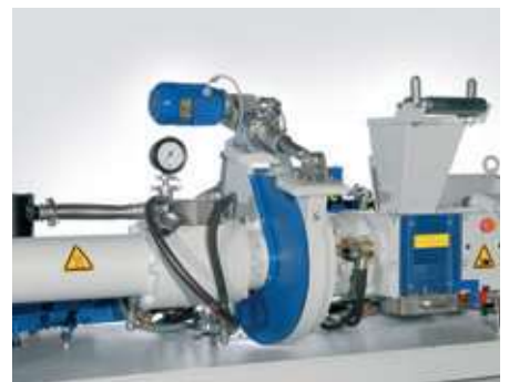
Hydraulically adjustable Pinconvert element
