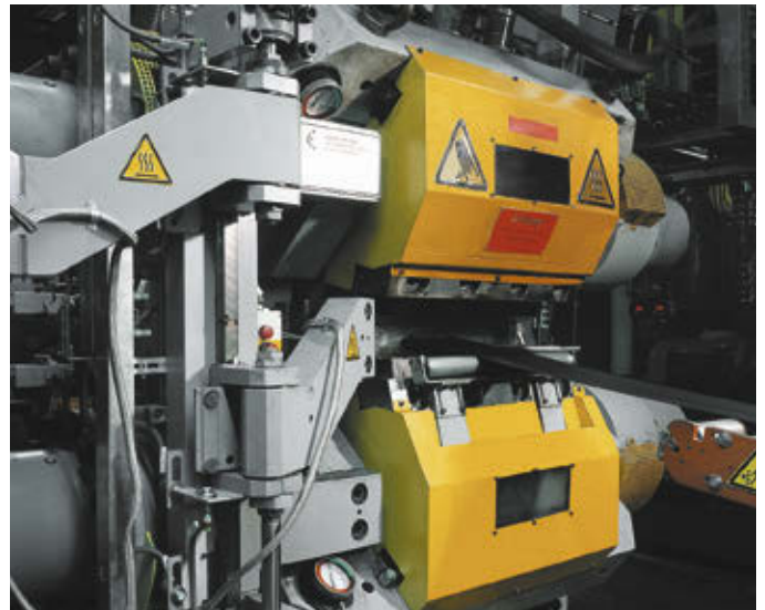
Multiplex extrusion head with cassette changer unit
