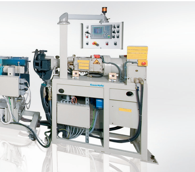
Extrusion line for the production of silicone hoses
