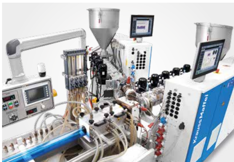
Production line of light strip profiles made of polycarbonate in the coextrusion process
