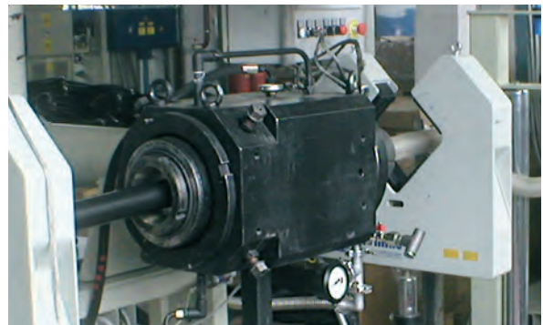
Extrusion die for sheathing the reinforcement
