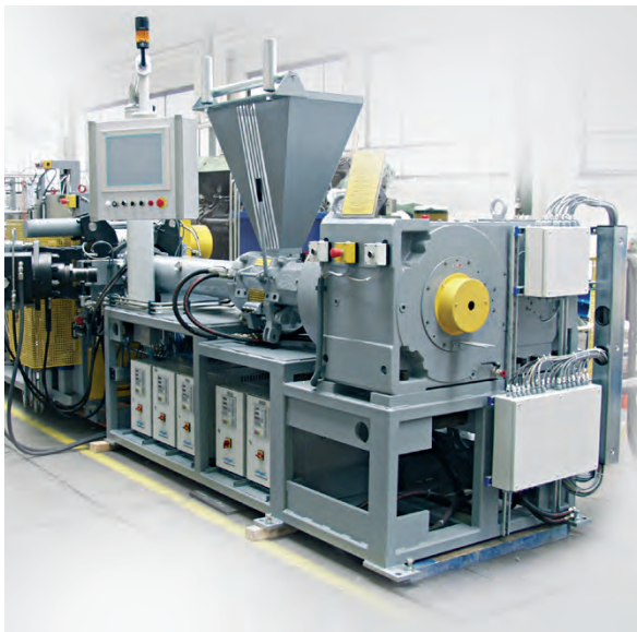
GE-K extruder for rubber hose production
