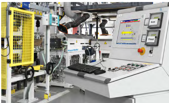
The entire laboratory-scale line is monitored and controlled from the central operator station.
