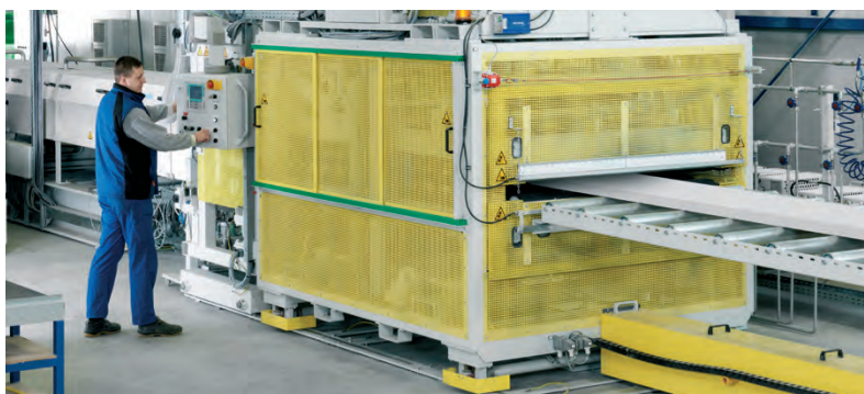
Plate calibrator of an ISO-BOARD Schaumtandex line
