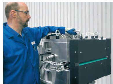
Customized slot die for board widths of up to 1,200 mm
