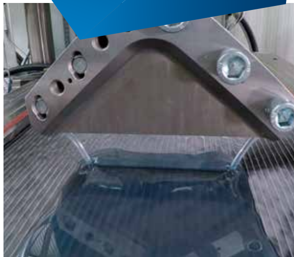
Flat sheet die: for both large-format and laminar application
