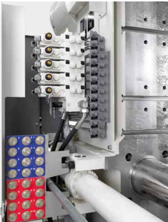
Easy media supply to the mold fixing platens
