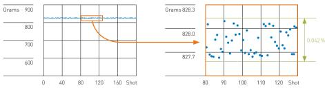
Shot weight consistency of 0.042% based on the example of a box lid with a shot weight of 828 g (PP) and a cycle time of 39 seconds.
